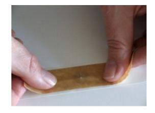
At the relevant point in your application process install the registration pin into the registration hole from the back of the mask.
