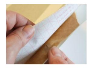
Each registration hole on a mask will require one of the above prepared registration pins installing.
