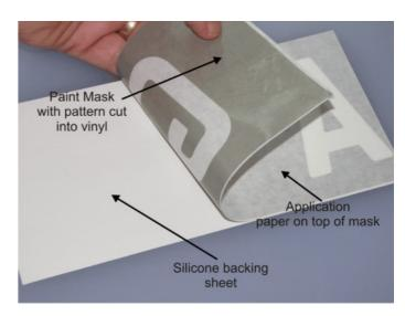
The masks can be used to apply detail to the model as long as the detail is not too fine. Single coloured markings such as serial numbers and aircraft letters are the easiest masks to use and the most critical thing to worry about is applying the mask in the correct position.
