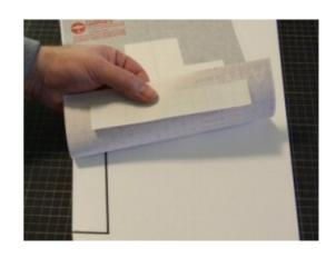
Once you have positioned your mask in the correct position, remove the silicone backing paper from the registration pin as shown opposite.
