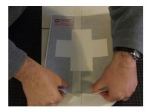
Lift the mask off and rub down the tape around the Registration pin to ensure it is securely located.
